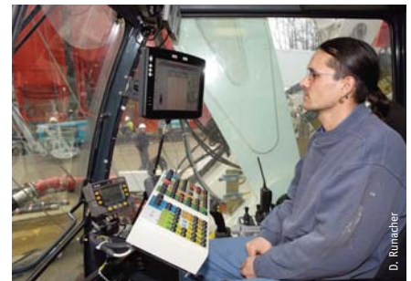
Hydrofraise driver's cab, equipped with the Enpafraise system
