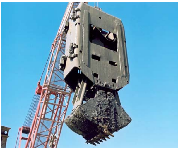
Self-guided cable grab. Sequential operation identical to that of the hydraulic grab.
