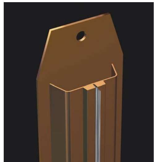
CWS process: temporary metal formwork supporting the water-stop sealing strip. This formwork is positioned at each end of the primary panels. The formwork is removed laterally after excavating the adjacent secondary panels.
