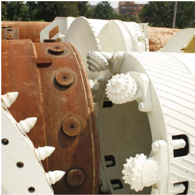
Hard rock coring tool with rotary cutters
