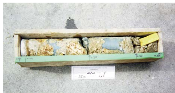
Record coring. The grey areas are the grouted porous zones.
