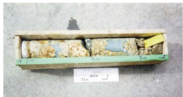
Record coring. The grey areas are the grouted porous zones.
